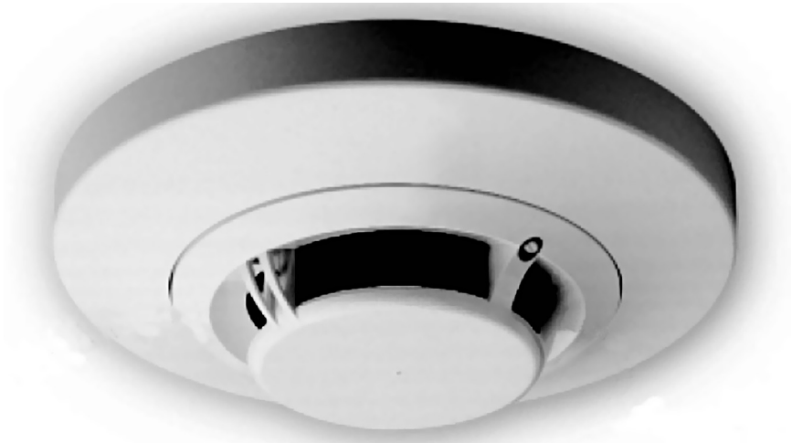
Figure 9.2 A Multicriteria Intelligent Sensor, Acclimate™ . This sensor incorporates both thermal and photoelectric technologies that interact to maximize detection. Acclimate is a fire sensor with an onboard microprocessor with advanced software that makes adjustments to reduce false alarms. Source: System Sensor.
