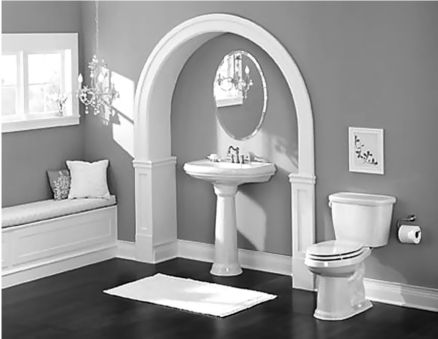
Figure 8.4 Certified by WaterSense, the Brienne High-Efficiency Toilet From Gerber Plumbing Fixtures Uses Just 1.28 gpf. The toilet also has a compact configuration, a FluidMaster 400A fill valve, a 3-in. flush valve for quick bowl cleaning, dual-fed siphon jets, and a 2-in. glazed trapway.
