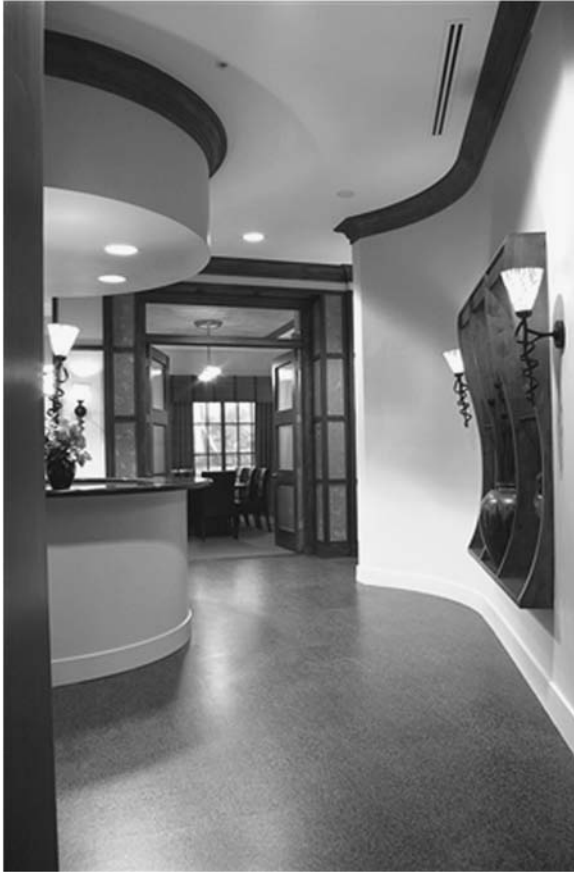
Figure 3.6 An Interior Space in Jupiter, Florida. It illustrates the impact that a careful selection of furnishings and finishes can have on a project. Diligent choices were made, such as cork for a sustainable material for flooring and walls, low-volatile organic compound paints, natural lighting, reuse of furnishings, green cleaning, and maintenance of the interior. Source: Denise Robinette – www.healthylivinginteriors.com
