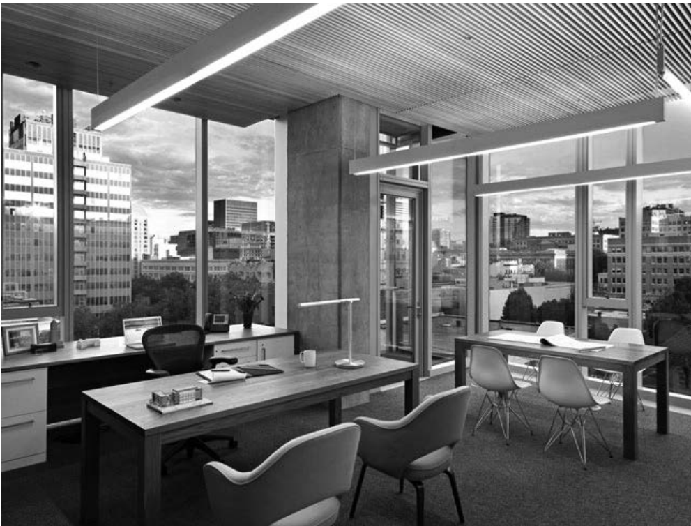
Figure 7. Lightly tinted glazing. The gray tint darkens the view but does not distort color balance, so it is acceptable vision glazing.
